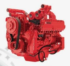
The original imported CUMMINS TIRE2 electronically controlled diesel engine. Single-stage turbocharging has good fuel economy and abundant power. Engine monitoring system can monitor the working condition of each cylinder in real time, prolong the service life of the engine and reduce the use cost. Advanced full-electronic control system adopts dual-electronic control module to ensure the best performance of the engine at different altitudes and loads.
